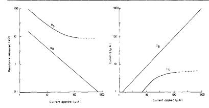
FIGS. 2A AND 2B. (A) The resistance of dry skin (R<sub>S</sub>) and skin submerged (R<sub>B</sub>) in Krebs-Ringer bicarbonate buffer, as a function of direct current, is measured by the four-point technique. (B) Currents through dry skin (I<sub>S</sub>) and submerged skin (I<sub>B</sub>) as a function of total applied current.
