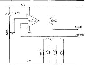
FIG. 1. Electrical circuit of the current source. The direct current is produced by a current source, which is supplied by two 9-V batteries. An operational amplifier ( $\mu$ P 741) assures each required current to be kept constant. The value of the output current is controlled by potentiometer (P) and range switch (S).
